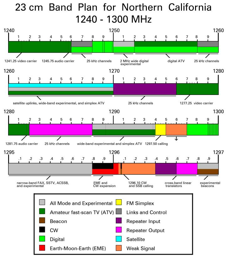
25 kHz spacing for narrow band channels as noted
